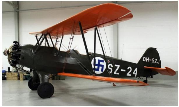
Less than 20 hours since a thorough, ground up restoration, including original Siemens SH-14 engine.
